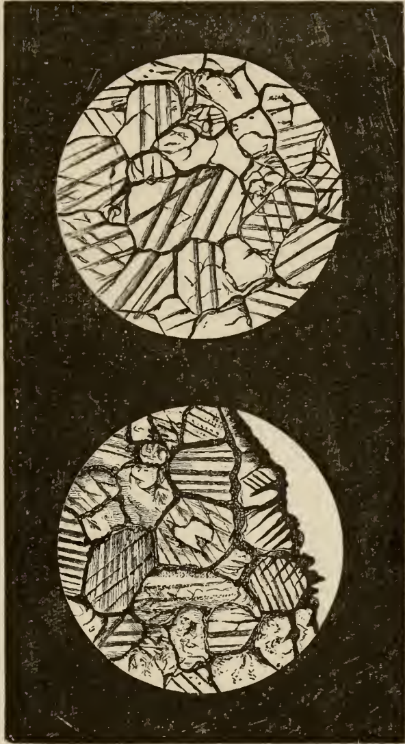
Fig. 24.—Microscopic structure of white marble employed in Edinburgh tombstones.
